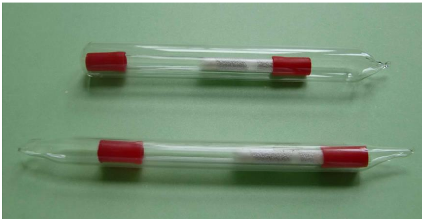
Fig. 6. Tube closed by plastic caps and flame-sealed in a glass tube (test tube).
