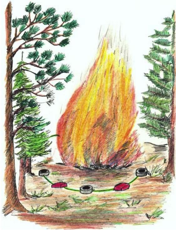
Fig. 2: Utilisation of the shock wave and negative oxygen balance by stoppage of the earthbound wildfire spreading
