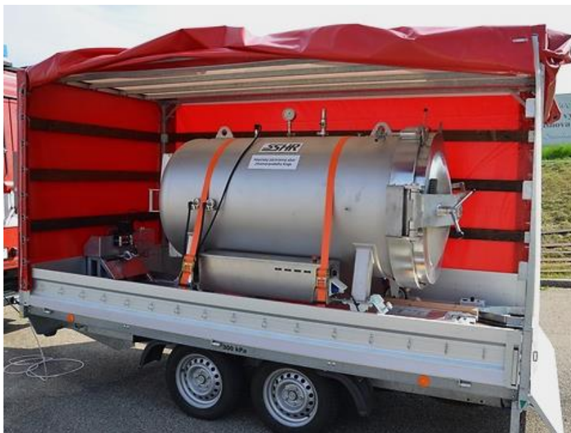
Figure 5 Gas-tight plenum chamber for the transport of dangerous cylinders
