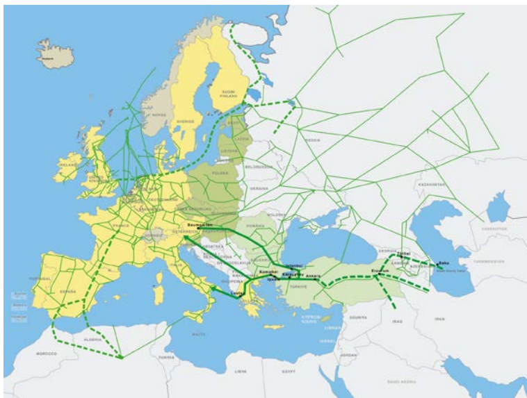
Fig. 1 Europe's natural gas pipeline network
